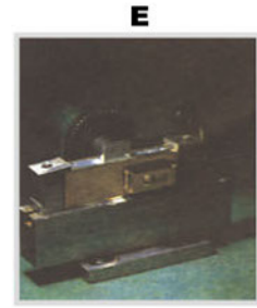
Lock Mechanism Life Cycle test for no. 5.
