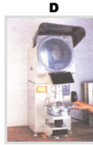
It is a Projected Use to Test Accuracy Dimension and Tolerance as well.
